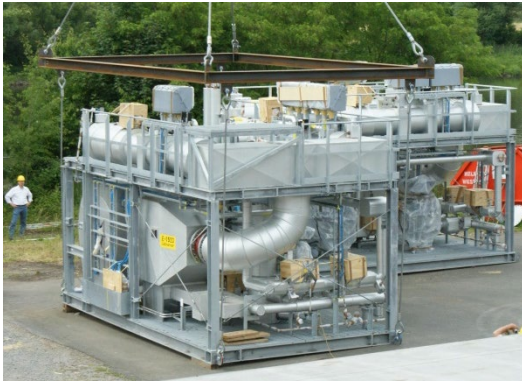
Aqueous ammonia vaporizer skids for refinery
