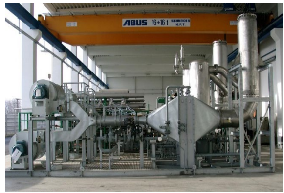
Aqueous ammonia vaporizer skids for coal power plant
