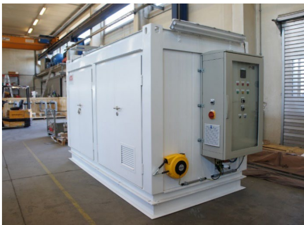
Mobile Steel Container PRMS with electrical heating and control panel: Flow: 2.500 nm 3 /h Pin: 20 – 200 bar Pout: 3 – 4 bar
