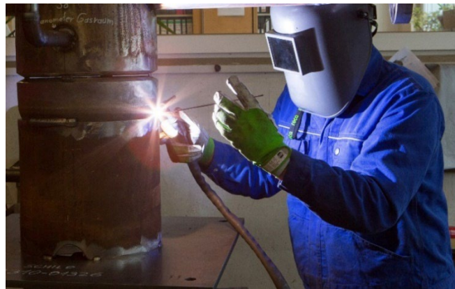
Welding of pressure vessel
