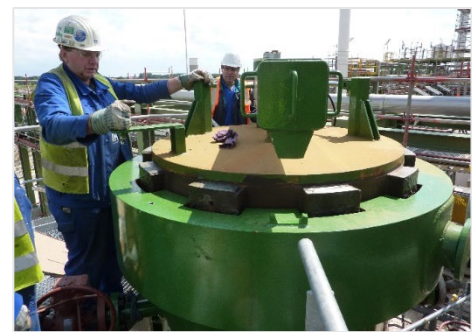
Quick Opening Closure DN 1300 (52"); PN300
