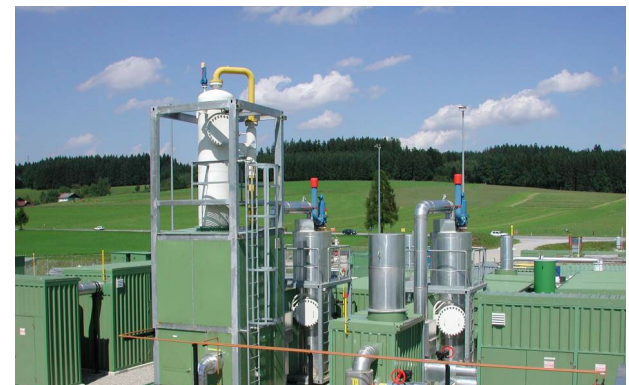
LTS unit gas production plant Gas flow: 1.000.000 nm 3 /d Pin: 40 – 70 bar TEG-flow: 1.000 kg/h
